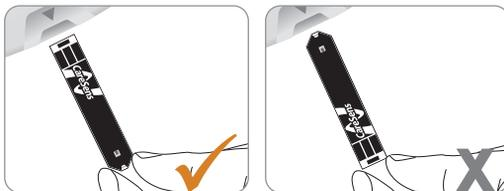
Insert a test strip with the contact bars facing upwards into the meter's test strip port. Push the strip in gently until the meter beeps. Be careful not to bend the test strip. The
