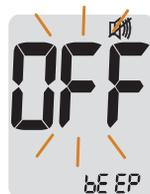
If the sound is set to OFF, none of the sound functions will work. After setting the sound, press the **S** button to progress to the next step.
